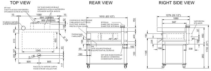
Nota: The dimensions indicated in the views are in millimetres. Steamer for Bakery only.
